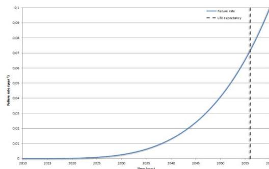
Figure 5 – Two-parameter Weibull distribution: failure rate  $\lambda(t)$  ( $\beta = 5$ ,  $\eta = 50$ )
