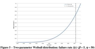
The 2-parameter Weibull distribution is not the most appropriate choice for describing the aging of all assets. This distribution imposes a zero failure rate at the beginning of the lifetime, which can introduce bias in the curves. A 3- or 4-parameter Weibull distribution would be more adapted in this
