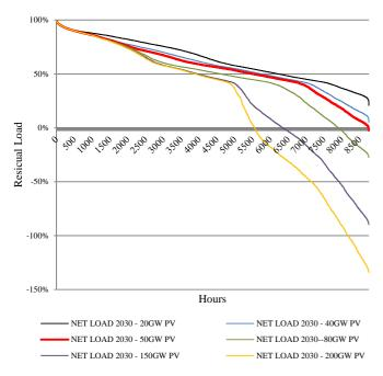
Figure 2: Residual load with different amount of PV generation capacities.
